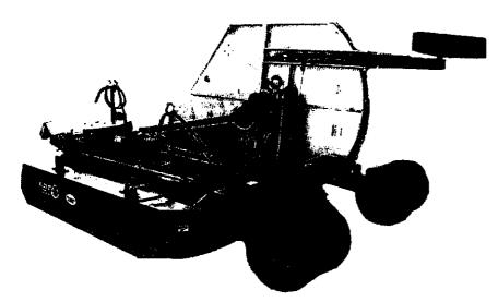
Deck rings and rear safety chains are standard equipment on the 10' Offset Flex Predator.
